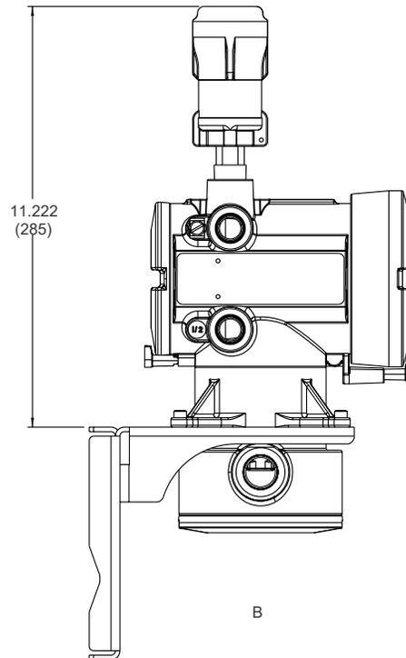
A. Remote-mount transmitter with integral-mount THUM Adapter
