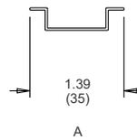
A. For mounting on a 1.39 in (35 mm) rail
