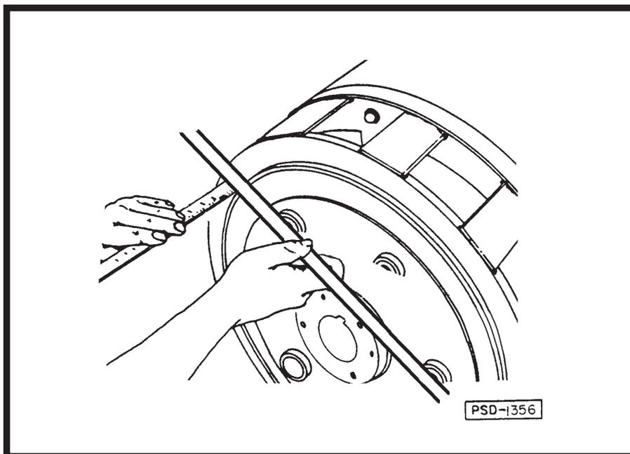
**Measuring from Mounting Face to Bushing**
