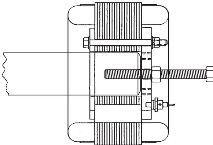
(Remove the 1/2-13 X 5-inch bolt and the nut after installing the exciter armature on the generator armature shaft.)
