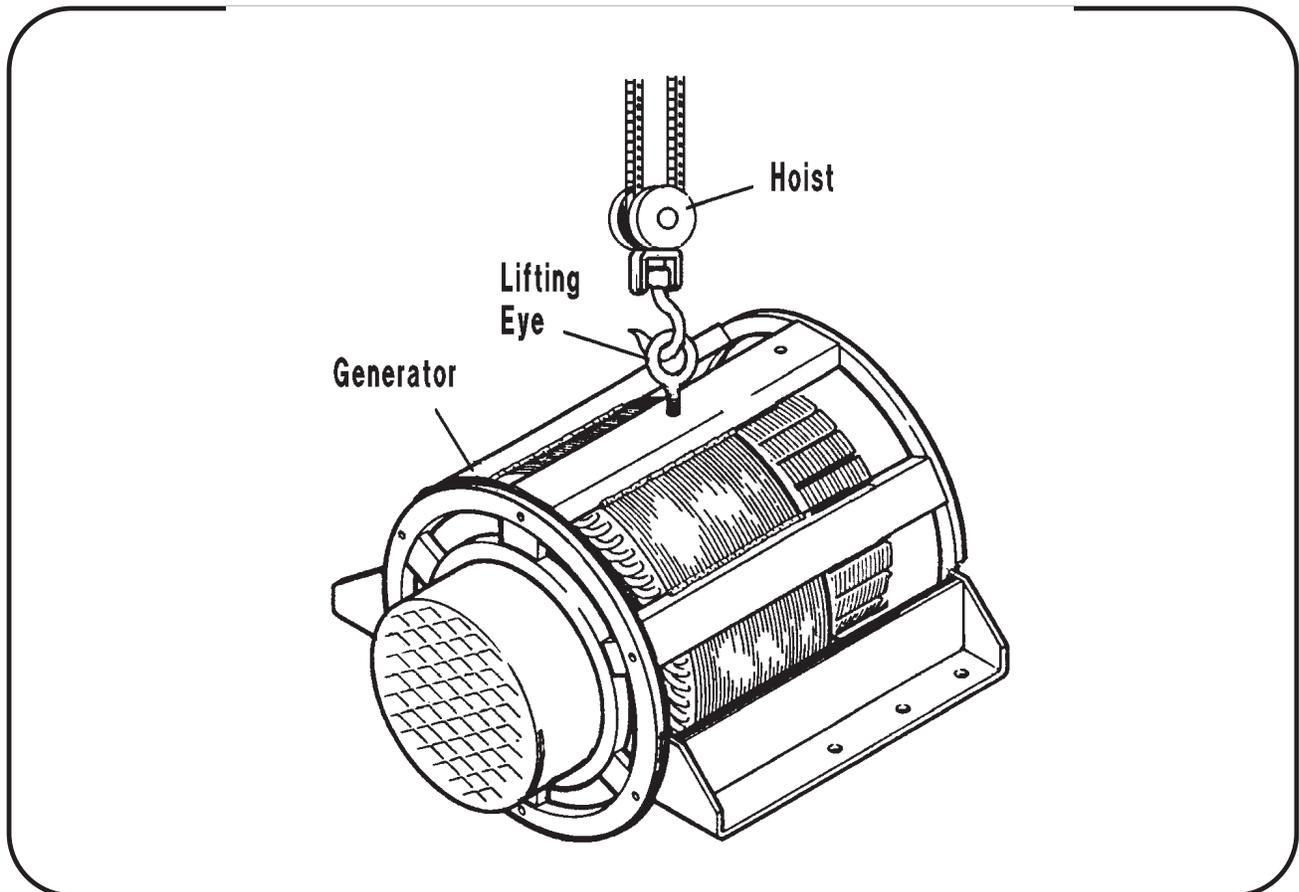
**Generator Lifting Arrangement**
